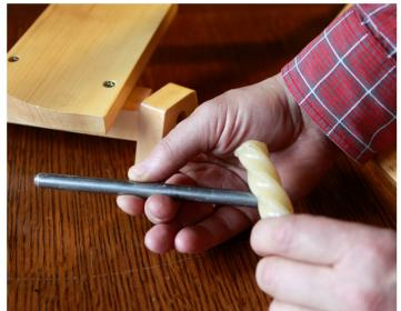
As it is shown in the picture, embrocate 1 - 2 minutes the thick bar connecting the treadles. It should be done carefully, to obtain thick layer of paraffin on the bar.
