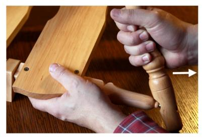
Step 1: Gain access to the parts that need to be lubricated by removing the treadle from one leg.
