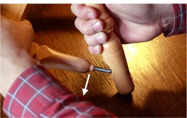
Once you have freed the pin from the cup inside of thr leg, guide the treadle pin to be in front of the leg.
